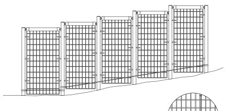
The welded grid panels can easily be modified to adapt to ground obstacles such as rocks and tree roots
